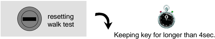
Fig. 7: Resetting all alarms and alarm devices
